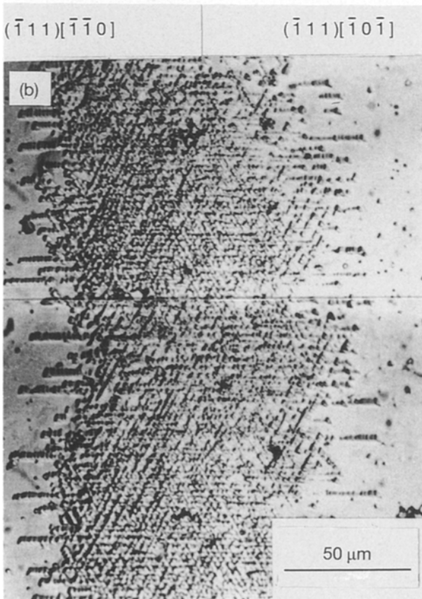
Figure 3 Appearance of etched surface. scratched direction: (a) [211] , (b) [2\bar{1}\bar{1}] .
